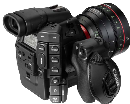
Handgrip attaches to camera right side, with buttons for start/stop, focus magnifier, and a dial to control iris of EF mount lenses. There are 2 CF Card slots at the rear. I recommend recording simultaneously to both: that provides a "camera negative" and a "backup dailies."
