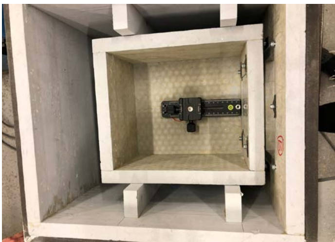
Fireproof box with silicate walls for Blackmagic Micro camera.
